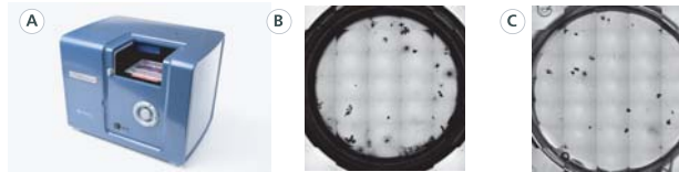
FIGURE 5: STEMvision™ Fully Automated CFC Assay Reader (A), Colony Image in Regular Dish (B) vs. Meniscus-Free SmartDish (C)
