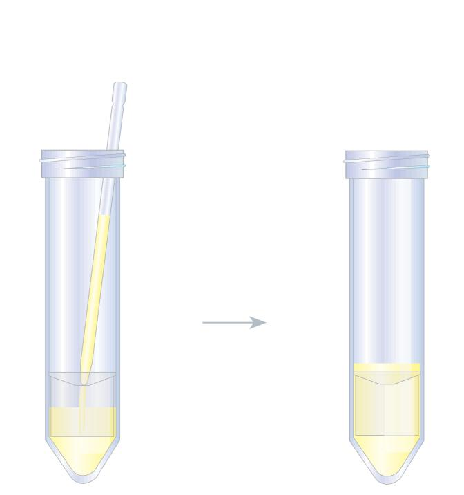
Add density gradient medium (e.g. Ficoll-Paque™ PLUS) to the SepMate™-50 tube by pipetting it through the central hole.
