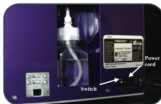
Figure 9 – Side view of RoboSep™ showing power and data connections, as well as the hydraulic fluid bottle and power switch.
