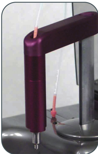
Figure 4 – The robotic arm is capable of vertical and rotational motion. The stainless steel tip head at the end of the arm is used to pick up pipette tips.
